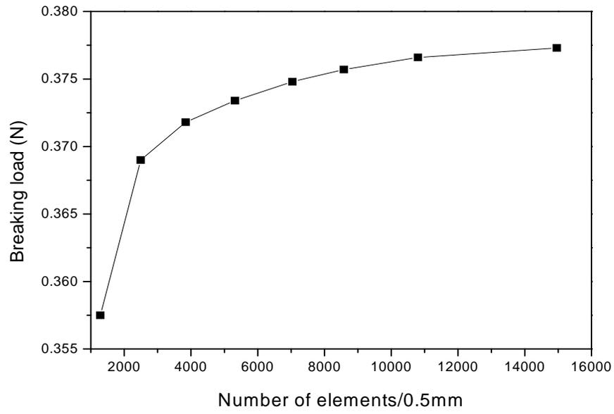
Figure 3: The breaking load versus number of elements (strain rate of 30,000%/sec)
