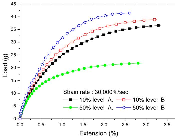
Figure 9: Load-extension curves for fiber with different diameter variation and position of the thinnest segment at the strain rate of 30,000%/sec
