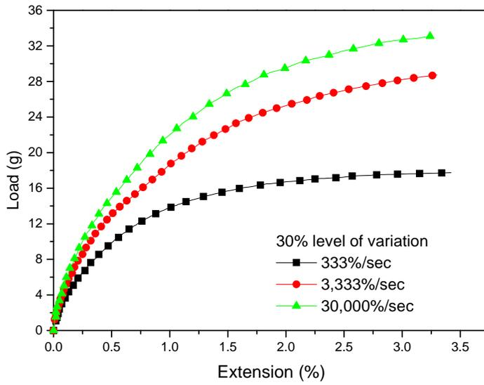
Figure 7: Load-extension curves for fiber specimen at different strain rates
