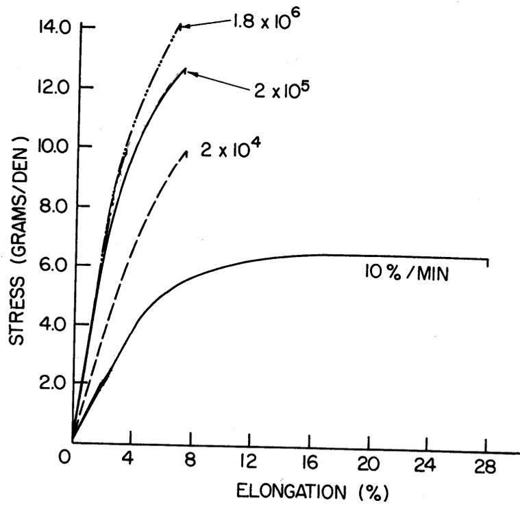
Figure 1: Stress-strain curves of polyethylene fibers at various strain rates <sup>1</sup>
