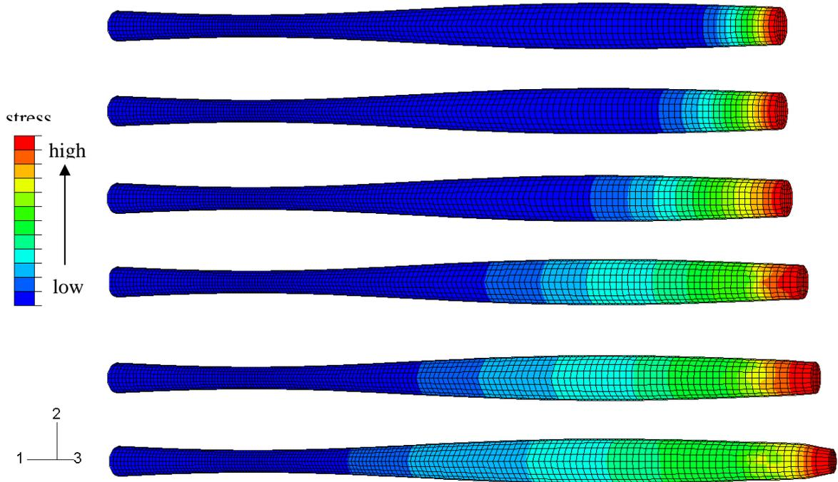
Figure 8: The contours of the stress in a fiber during successive extensions
