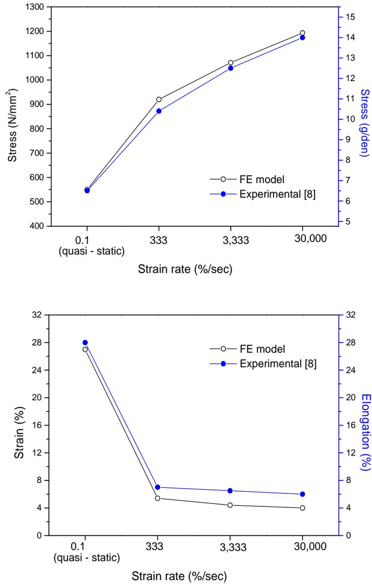
Figure 4: Comparison of the simulation results from FE model and experimental results obtained by Lyons under quasi-static condition and at three different strain rates
