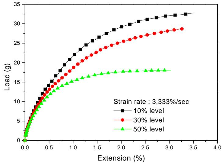
Figure 6: Load-extension curves for fiber specimen with different levels of diameter variation (strain rate of 3,333%/sec)
