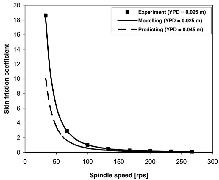
Figure 2 Modeling of skin friction coefficient on a package surface for YPD (yarn package diameter) = 0.025 m and predicting for YPD = 0.045 m.
