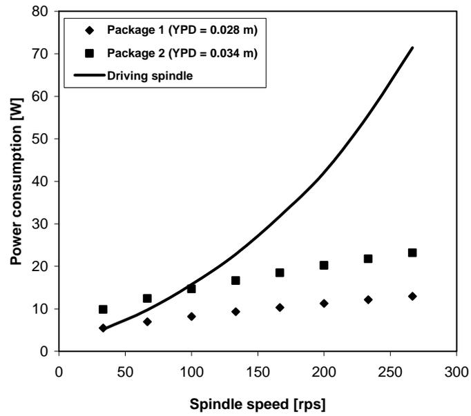
Figure 3 Comparison of powers consumed on overcoming skin friction drag and driving spindle during yarn winding.
