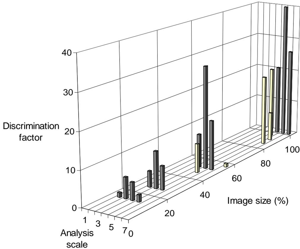
**Figure 2.** Discrimination factors obtained for all analysis scales that produced a feasible analysis basis for all image sizes - 1840 double jersey series
