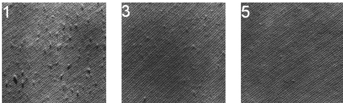
**Figure 1.** Standard pilling test images - 1840 double jersey series
