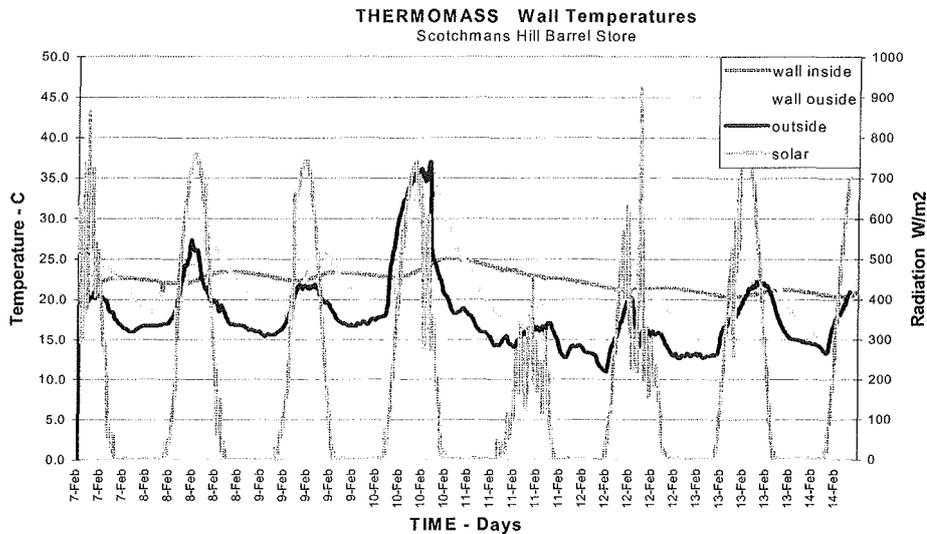
Figure 4 Charted Wall Temperatures of the THERMOMASS panel alongside external conditions
