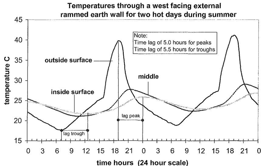
**Figure 3 In-situ Time Lag Testing of a 300mm Rammed Earth Wall**
