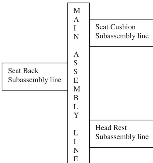
Figure 2: Front seat assembly block diagram
