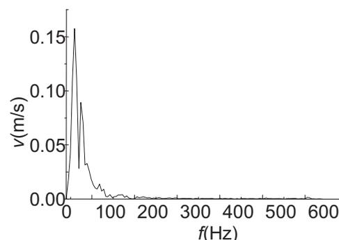
Fig 2. Seismic frequency spectrum of gasoline engine vehicle
