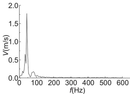
Fig 3. Seismic frequency spectrum of heavy diesel engine vehicle
