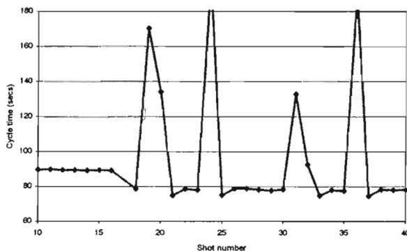
Figure 4. Cycle time during first trial on the converter housing
