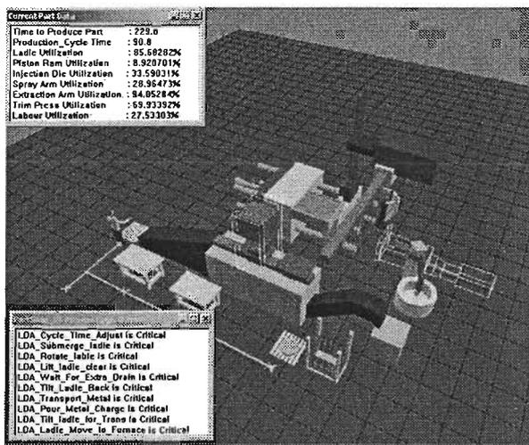
Figure 1. Timing model showing utilisation levels and critical path.
