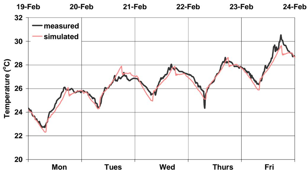
**Figure 5 Simulated and measured office air temperatures**
