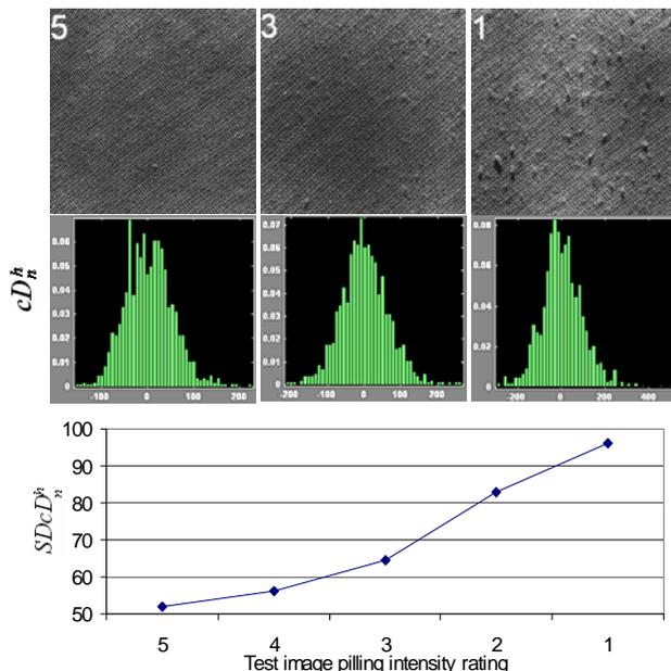
Fig. 1. (top) James H. Heal '1840 double jersey' fabric test images, (centre) Distribution of 2DDWT detail coefficients, and (bottom) Standard deviation of wavelet detail coefficients
