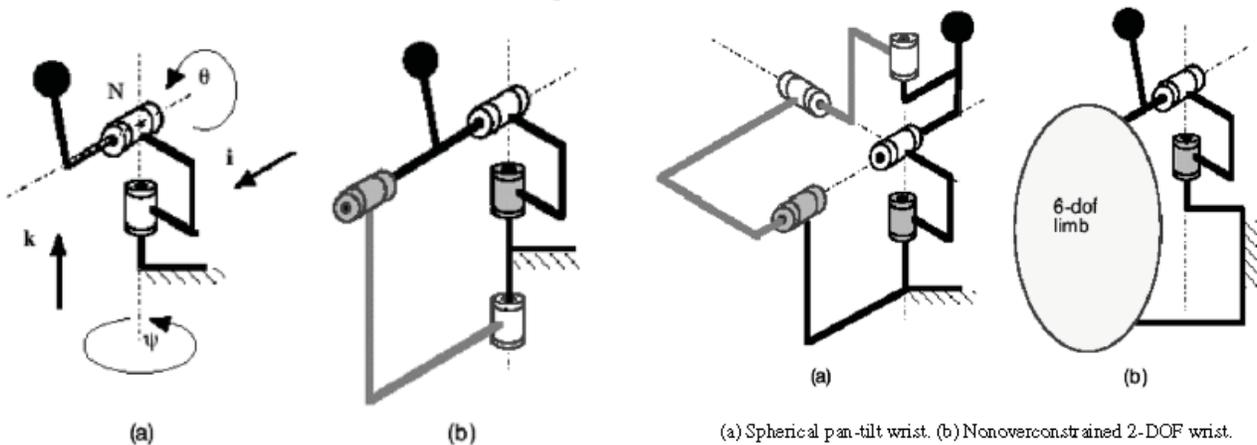
(a) Serial pan-tilt wrist. (b) Parallel pan-tilt wrist.
