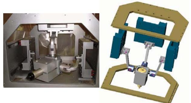
**Figure 7 - Industrial-Scale Three DOFs Head**
