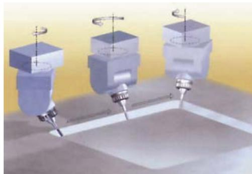
Figure 3 - Machine Geometry/Kinematics demands high joints speed and acceleration
