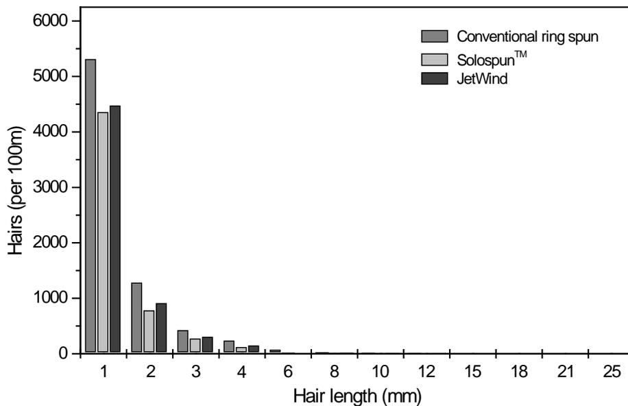
Figure 3. Comparison of the number of hairs normalised to 100 meters for the conventional ring spun, Solospun<sup>TM</sup> and JetWind yarns.
