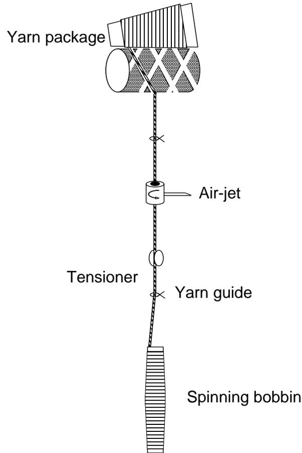
Figure 2. Schematic diagram of the JetWind process.
