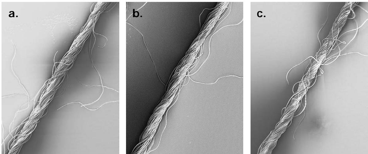
Figure 4. Representative illustrations of the hairiness characteristics of a). conventional worsted spun yarn, b). Solospun<sup>TM</sup> spun yarn, and c). ring spun yarn processed via JetWind set-up
