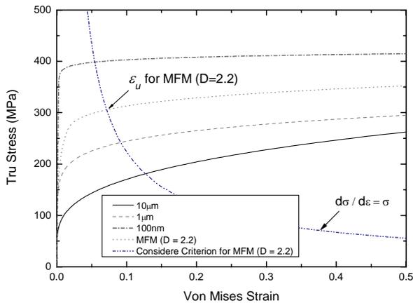
**Figure 4.** True stress – strain curves for pure copper with different microstructures:  $d = 100$  nm,  $1$   $\mu$ m,  $10$   $\mu$ m, and fractal microstructure with  $D = 2.2$ .
