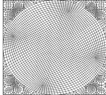
**Figure 3.** Typical mesh of three-phase unit cell model for  $D = 1.4$ .
