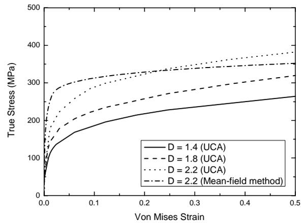
**Figure 8.** The true stress-strain relations of pure copper with three-grain microstructures at fractal dimension  $D = 1.4, 1.8$  and  $2.2$ .
