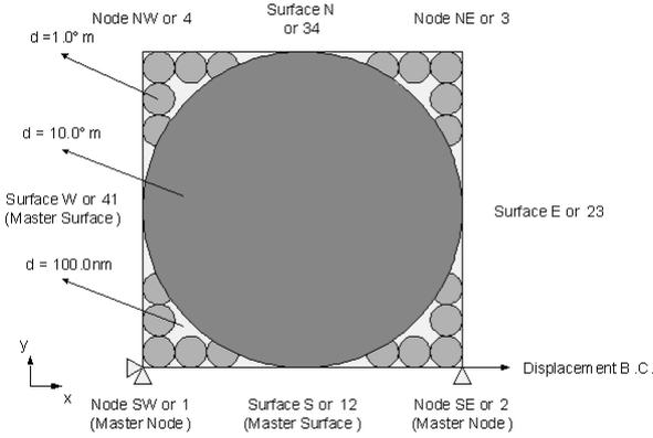
**Figure 1.** Three-grain unit cell model of MMC with the periodicity boundary conditions.
