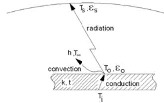
Figure 3. Through the refractory, heat transfer takes place by conduction, free convection, and radiation.
