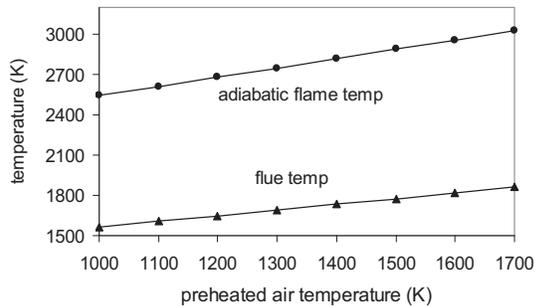
Figure 4. Variation of adiabatic flame temperature and furnace flue temperature with respect to preheated air temperature.
