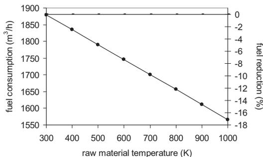
Figure 6. The absolute and relative values of fuel consumption with respect to raw material temperature.
