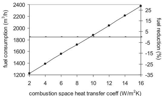
Figure 7. The absolute and relative values of fuel consumption with respect to  $U_{\text{combustion space}}$ .
