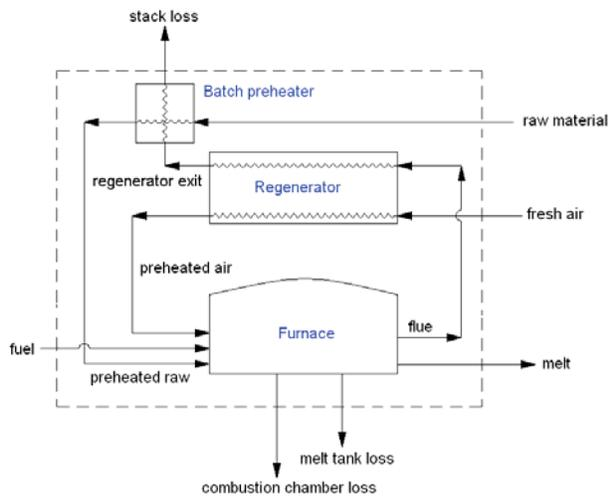
Figure 1. The control volume of a glass melting plant.
