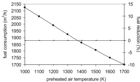
Figure 5. The absolute and relative values of fuel consumption with respect to air temperature.
