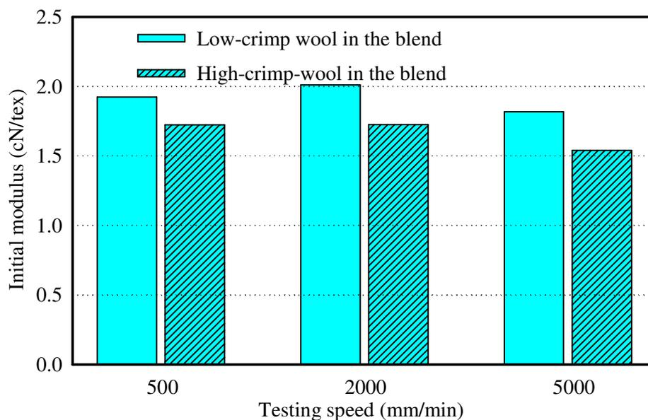
**Figure 5** Initial moduli of alpaca/wool blend yarns at different tensile testing speeds
