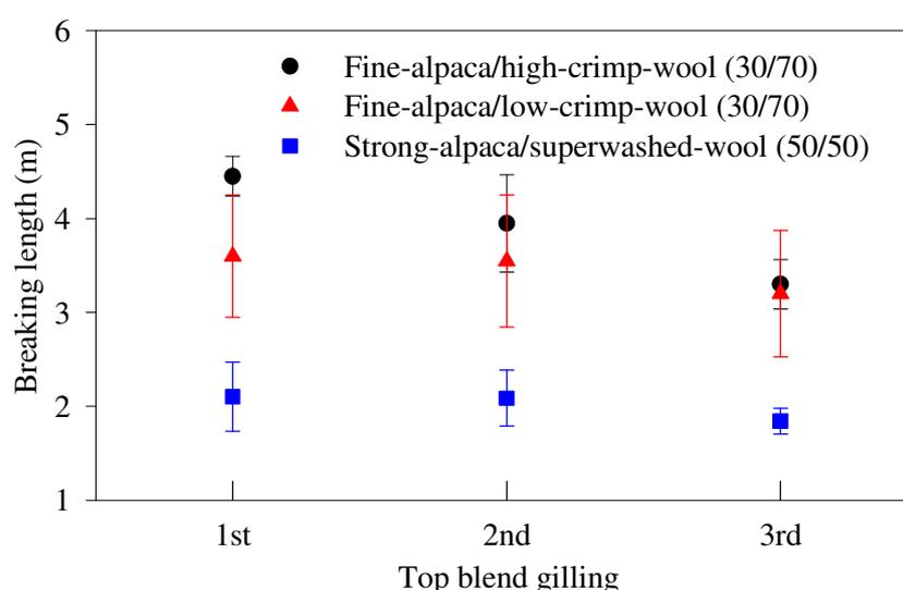
**Figure 2** Breaking length of slivers of alpaca/wool blends at different blending passages
