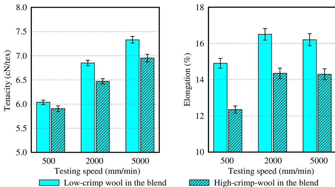
**Figure 4** Effect of tensile testing speed on the tensile properties of alpaca/wool blend yarns
