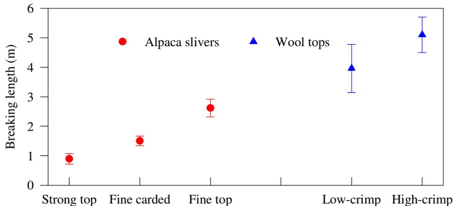
Figure 1 Breaking length of different slivers
