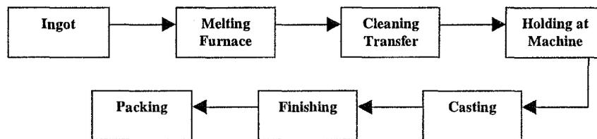
Figure 1. Die casting process
