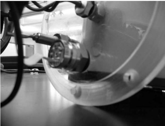
**Fig. 5 Photograph of Mounted Pressure Transducer**
