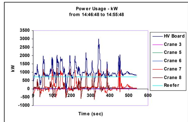
Fig. 7. Power curves – snap shot of power usage of the substation
