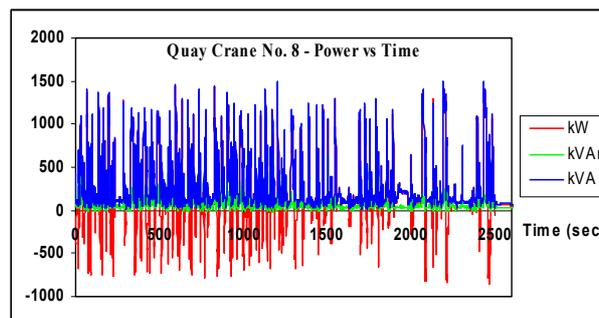
Fig. 5. Quay crane No.8 – Captured 1 second data – Graph of powers vs time.
