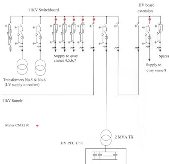
Fig. 3. Supply arrangement of substation
