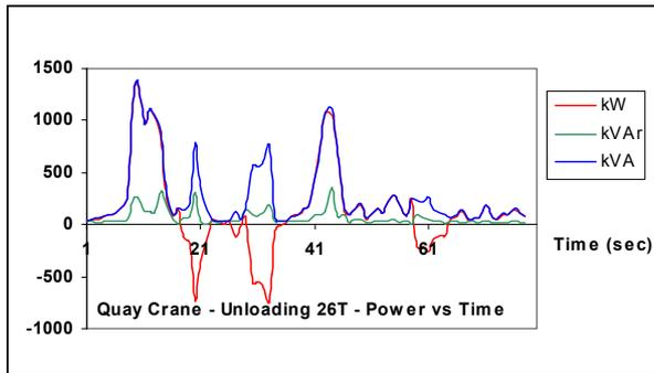
Fig. 6. Quay crane No. 8 – Captured 1 second data – Graph of powers vs time for one loading cycle: Lock container – Hoist – Hoist & Cross travel – Lower – Unlock container – Hoist – Hoist & Cross Travel – Lower & land on top of next container.
