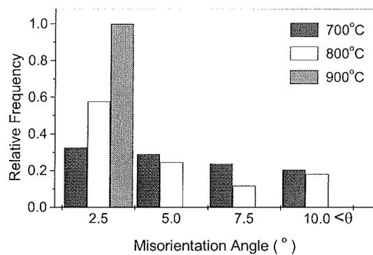
Figure 3: The misorientation angle distribution as a function of deformation temperature at a strain of 1 for the Ni-30Fe alloy [9]
