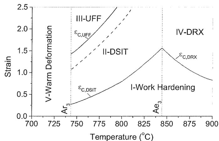
Figure 1: Microstructural map for 0.17C-1.5Mn-0.02V (in %wt) steel at strain rate of  $1 s^{-1}$  and cooling rate of  $3 °C/s$  for austenite grain size of  $84 \mu m$  (broken line represents  $\epsilon_{C,UFF}$  at cooling rate of  $5 °C/s$ ) [8]
