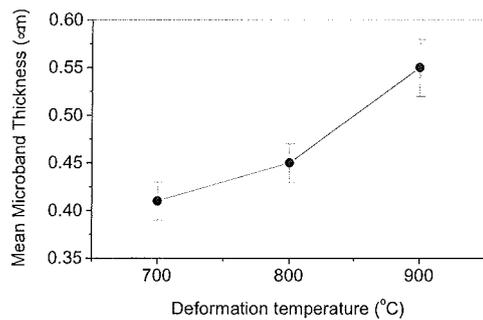
Figure 2: Mean microband thickness as a function of deformation temperature at strain of 1 and strain rate of  $1s^{-1}$  for the Ni-30Fe alloy [9]
