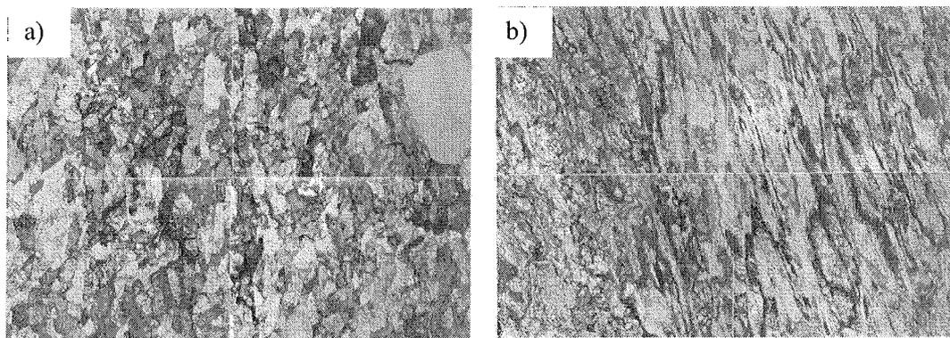
Figure 4: Microstructures of Ni-30Fe alloy at different deformation temperature at 70% reduction: a)  $800^{\circ}\text{C}$  and b)  $530^{\circ}\text{C}$  [11]
