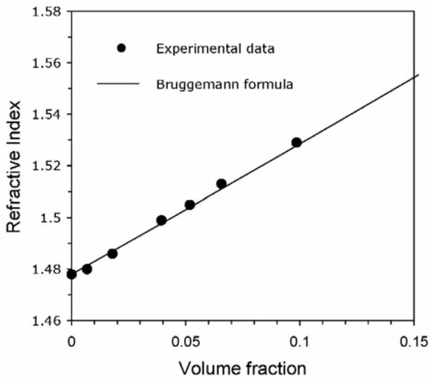
Figure 4. Refractive indices of ZnO / alkyl benzoate hybrid films.
