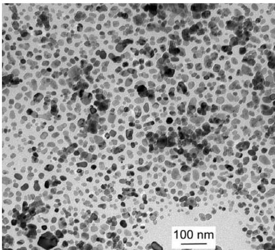
Figure 1. Transmission electron microscopy image of ZnO nanoparticles coated with stearic acid.
