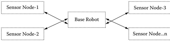
**Figure 14.5** Base robot and sensor network communication—star configuration.
