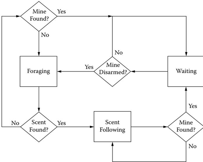
Figure 14.9 Flow chart of the implemented swarm algorithm.
