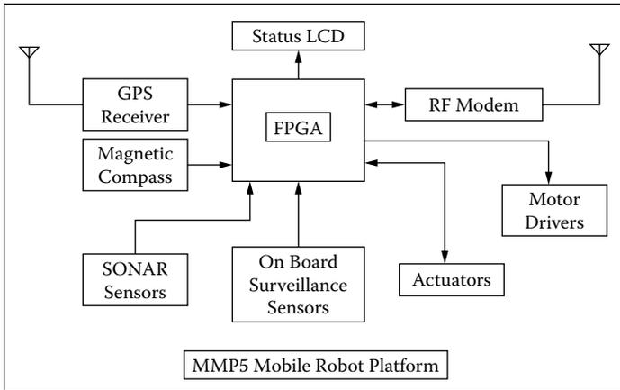
Figure 14.6 Architecture of the robot.
