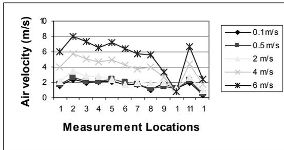
**Figure 4:** Air velocity within the canyons at different wind speeds.
