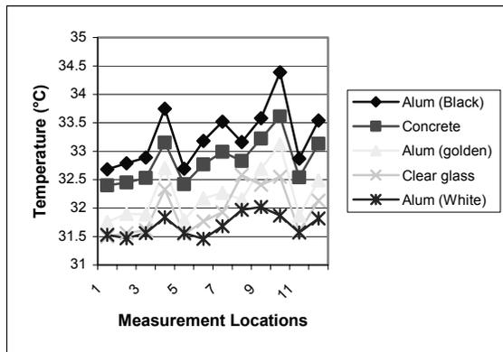
**Figure9:** Air temperature inside the canyon using different façade materials
