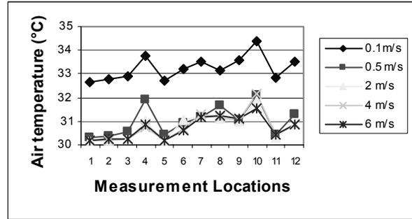
**Figure 5:** Temperature within the canyons at different wind speeds
