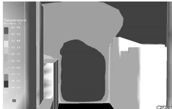
**Figure 7:** Temperature contours at location11 for black Aluminium at wind speed 2m/s
