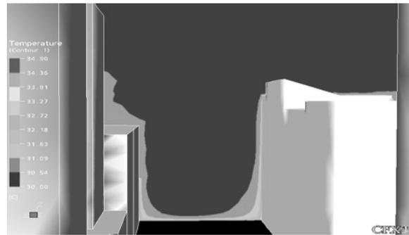
**Figure 6:** Temperature contours at location11 for black Aluminium at wind speed 4m/s
