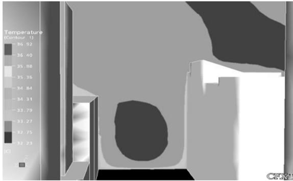
**Figure 8:** Temperature contours at location 11 for black Aluminium at wind speed 0.1m/s
