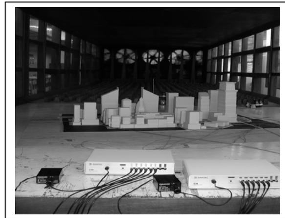
**Figure 2:** Model used for wind tunnel experiment
