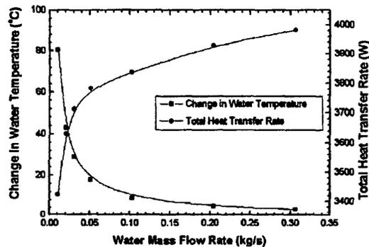
Figure 8. Variation in water temperature and total heat transfer rate with coolant flow rate
