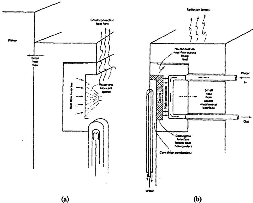
Figure 1. Heat paths available in HPDC. (a) Die open for service (b) Die closed after shot [2]
