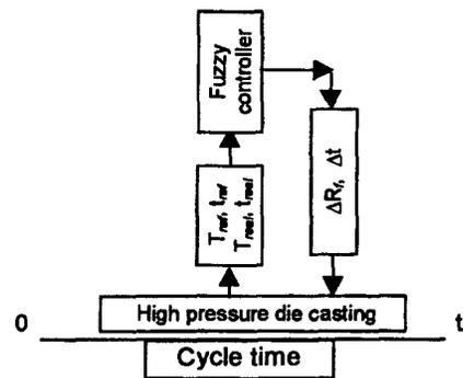
Figure 7. Adaptive fuzzy controller for high pressure die casting
