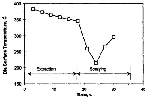
Figure 6. Variation in die temperature when die is open
