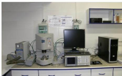
**Figure 3.** Rotation/vibration rheometer for characterization of flow properties of polymer melts.
