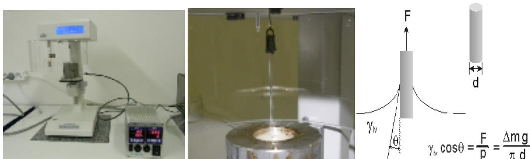
**Figure 2.** Measuring method for characterization of the surface tension of polymer melts.
