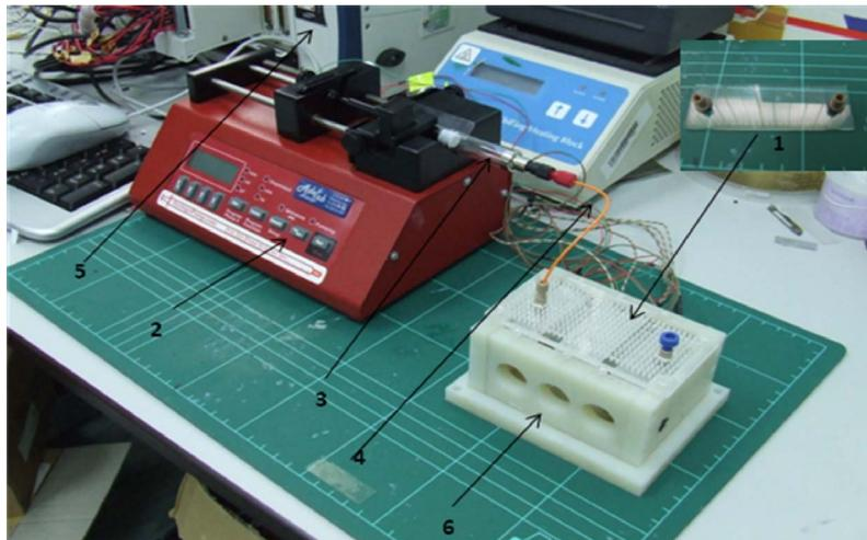
FIG. 4. PCR chip system setup. (1) PCR glass chip, (2) syringe pump, (3) glass syringe, (4) fluidic connections, (5) temperature control system, and (6) heater housing with temperature sensors.
