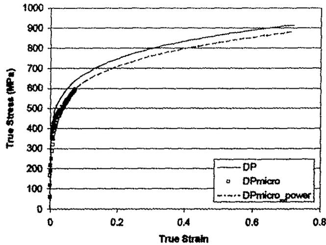
**Figure 10 Flow curves of DP and DP micro with fitted power law**
