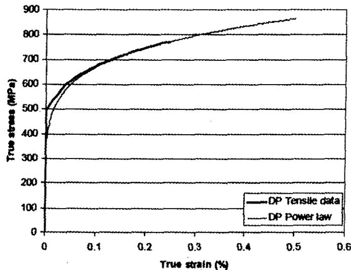
Figure 3 Experiment true stress-strain curves fitted with the power law for DP steel
