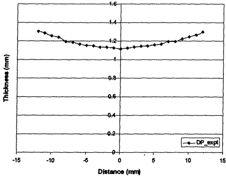
Figure 5 Experimental thickness distribution measured over the dome
