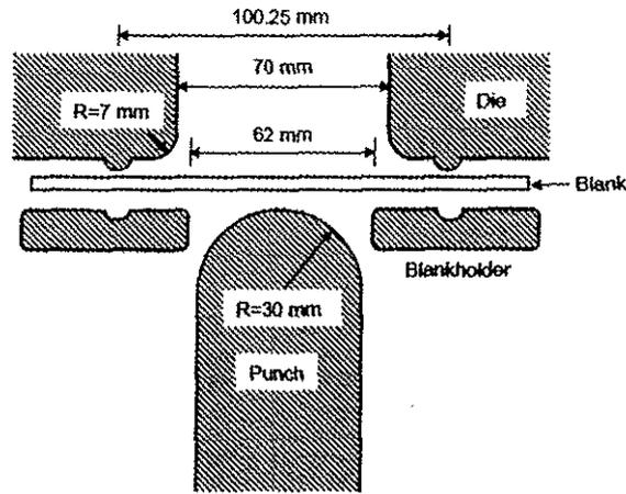
Figure 1 Experimental set-up of Erichsen stretch forming
