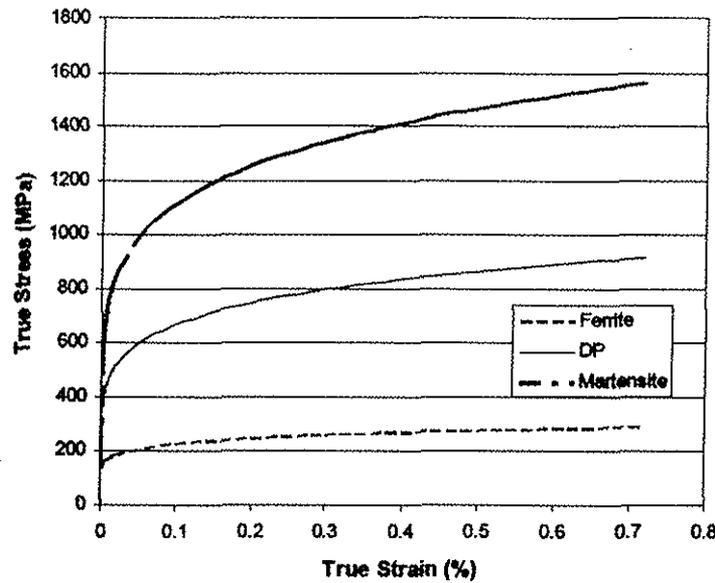
Figure 8 Flow curves for Ferrite, Martensite and DP steel
