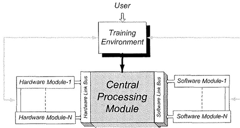
Fig 1. HIVEx System Architecture
