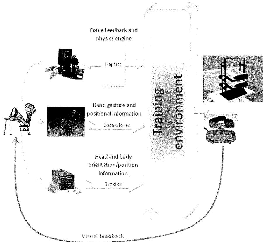
Fig 2. Hardware interaction involved in HIVEx System
