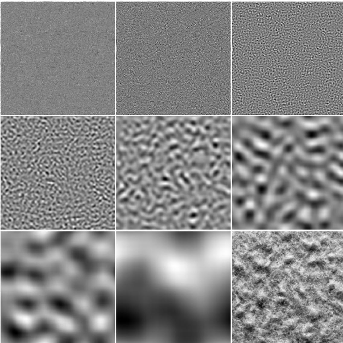
Figure 2. Reconstructed scale 1 to 7 detail images and scale 7 approximation image of pilling grade 1 nonwoven sample image by 2DDTCWT
