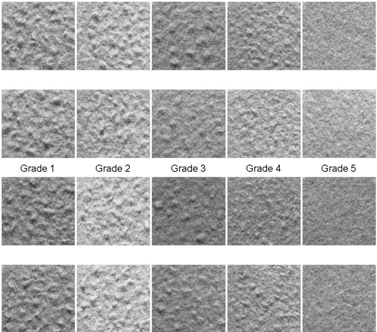
Figure 1. Prepared image samples from the WoolMark® standard nonwoven pilling test image set
