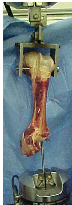
Figure 1 An Ox femur is mounted on the servo-hydraulic material test system.
