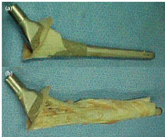
Figure 2 Failure at the (a) prosthesis-cement and (b) cement-bone interfaces.
