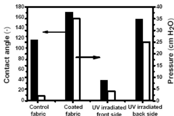
FIGURE 3. Water contact angles and breakthrough pressures on the fabrics
