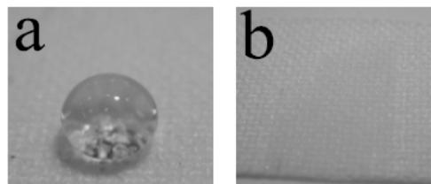
FIGURE 1. Water drops on (a) coated, and (b) pristine polyester fabrics
