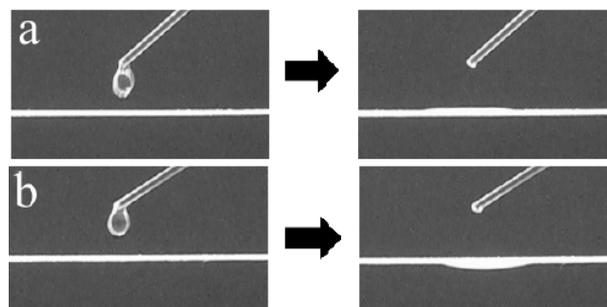
FIGURE 2. Photos of dropping water on the treated polyester fabric. (a) Upper surface was UV treated, (b) down surface was UV treated.
