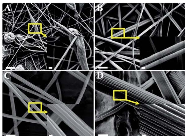
**Fig. 1** CAB fibres electrospun from (A) 5 wt%, (B) 12 wt%, (C) 15 wt%, and (D) 30 wt% (grams in 100 ml solvent) CAB solutions (solvent, acetone/DMAc = 2/1, v/v). Scale bar (main picture) = 2  $\mu$ m, scale bar (inset) = 200 nm.
