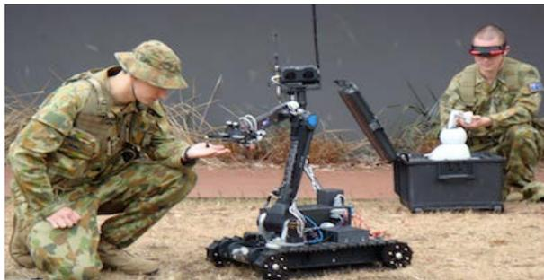
**Figure 5:** The OzBot setup with the capability of haptics and remote operation [9].
