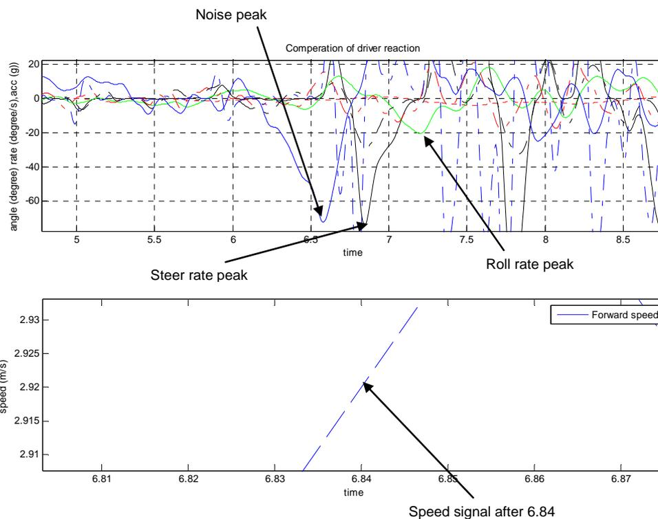
Figure 6: Signal responses after a disturbance (28)
