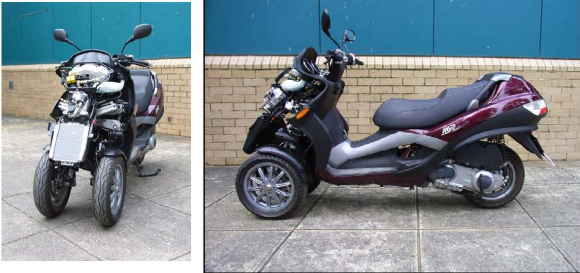
Figure 7: MP3 tilting system replaced with Saferide™ system with hydraulic cylinders, front and side view.
