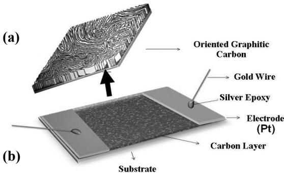
Figure 5. Schematic diagrams of the (a) oriented carbon film and (b) fabricated sensor with Pt contacts.
