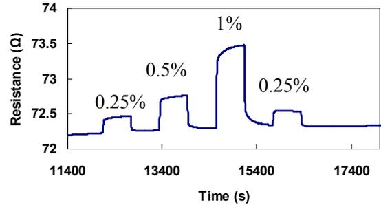
Figure 6. Dynamic responses of the sensor in the presence of various indicated hydrogen concentrations in synthetic air at 100 °C.
