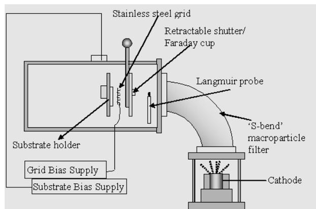
Figure 1. Schematic diagram of the biased grid and sample holder within the FCVA deposition system.
