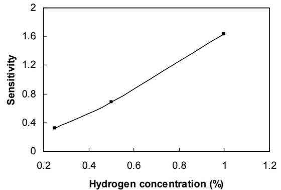
Figure 7. Percentage change in resistance(sensitivity) upon exposure the sensor to different hydrogen concentration at 100 °C.
