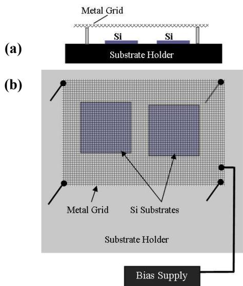
Figure 2. Schematic (a) cross section and (b) plan view diagrams of the substrate holder and the grid.
