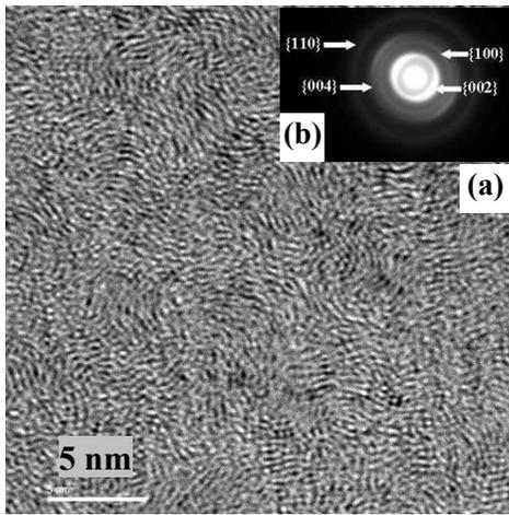
Figure 4. Schematic(a) High resolution TEM image and corresponding (b) selected area diffraction pattern from the carbon film prepared at 75 V bias and a substrate temperature of 400 °C using grid.
