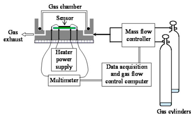
Figure 3. Schematic diagram of gas sensing test apparatus.
