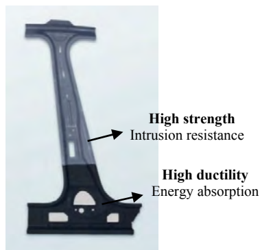
Fig. 1 A sample B-Pillar with tailored mechanical properties
