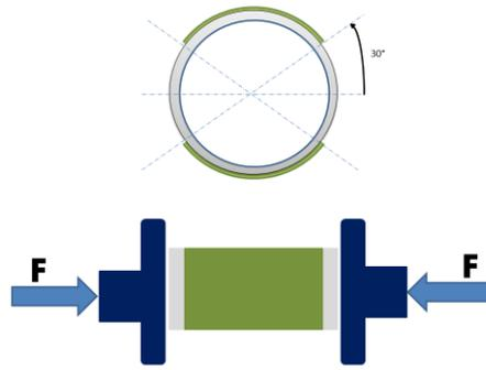
Figure 2 ASTM G70 – 07 test method for horizontal bending/ovalization aiming to evaluate coating flexibility.
