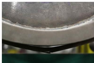
Figure 4 “Peaking” occurred when a mandrel is pressed on a specimen of 5 mm of steel coated with FBE.
