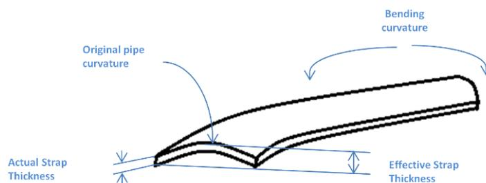
Figure 3 NACE standard RP0394-2002 pipe specimen schematic figure.
