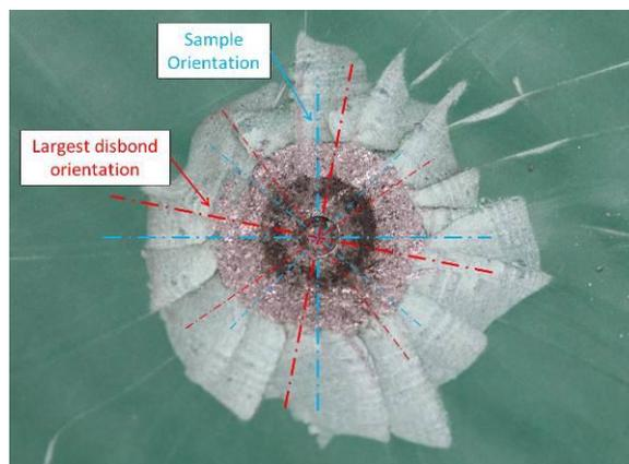
Figure 7 The disbondment radius measurement may vary the result.
