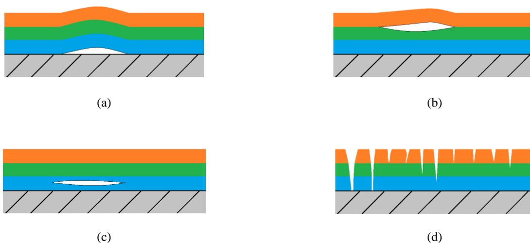
Figure 1 Adhesive and cohesive failure forms: (a) loss of adhesion to the substrate; (b) loss of adhesion to another type of coating; (c) horizontal loss of cohesion on one of the coatings; (d) vertical loss of cohesion of one or more coatings.
