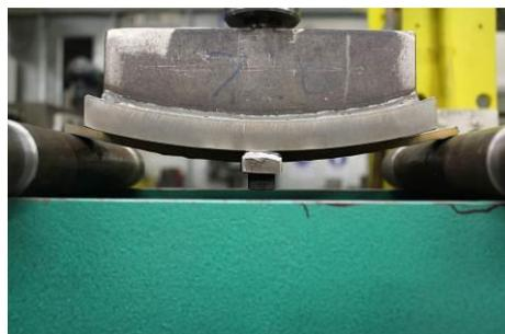
Figure 6 Solution for the “peaking” on samples using clamps.
