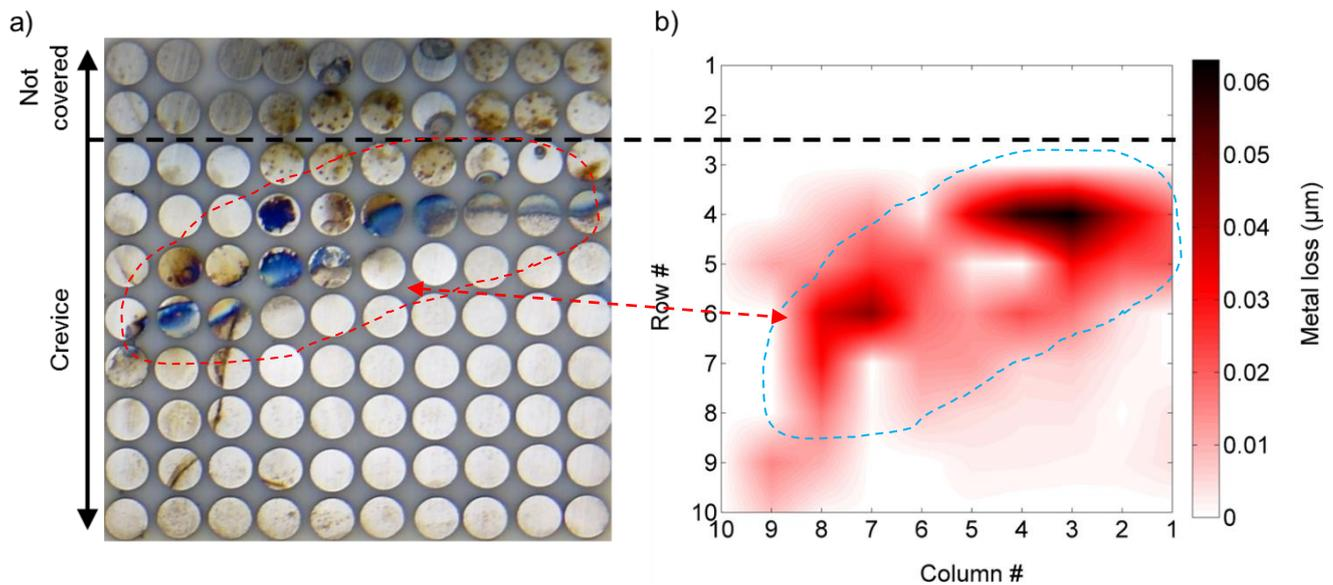
Figure 4. Comparison between actual (a) and measured (b) corrosion patterns.
