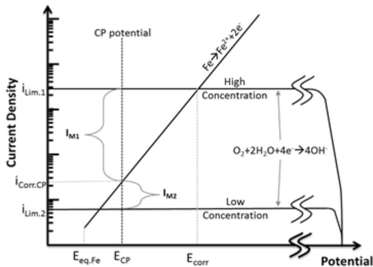
Figure 5. Schematic Evans's diagram of the probe's working principle.
