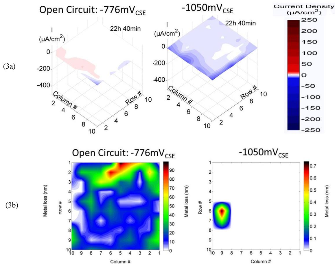
Figure 2. (a) Current density distributions over a sensor surface after 23hs exposure to 0.01M  $\text{Na}_2\text{SO}_4$  saturated sandy soil under OCP and under CP; (b) Metal loss maps calculated from the sensor's output under OCP and under CP respectively.
