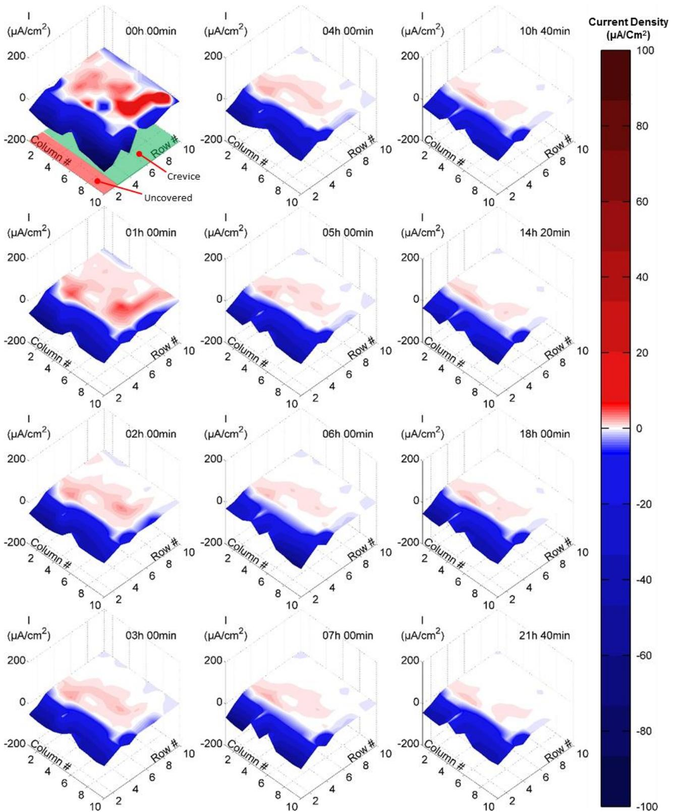
Figure 3. Current density distribution maps at several immersion times in 0.001M  $\text{Na}_2\text{SO}_4$  at  $-760\text{mV}_{\text{Ag}/\text{AgCl}}$ .
