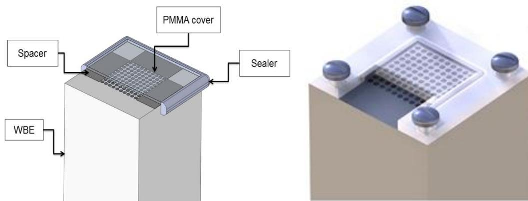
Figure 1. A novel sensor for simulating a disbonded coating over a simulated CP protected pipeline surface.
