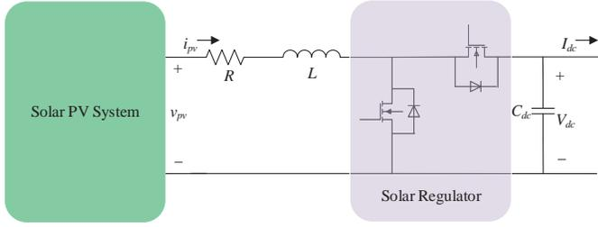
Fig. 5. Solar PV system with a solar regulator (DC-DC buck-boost converter)
