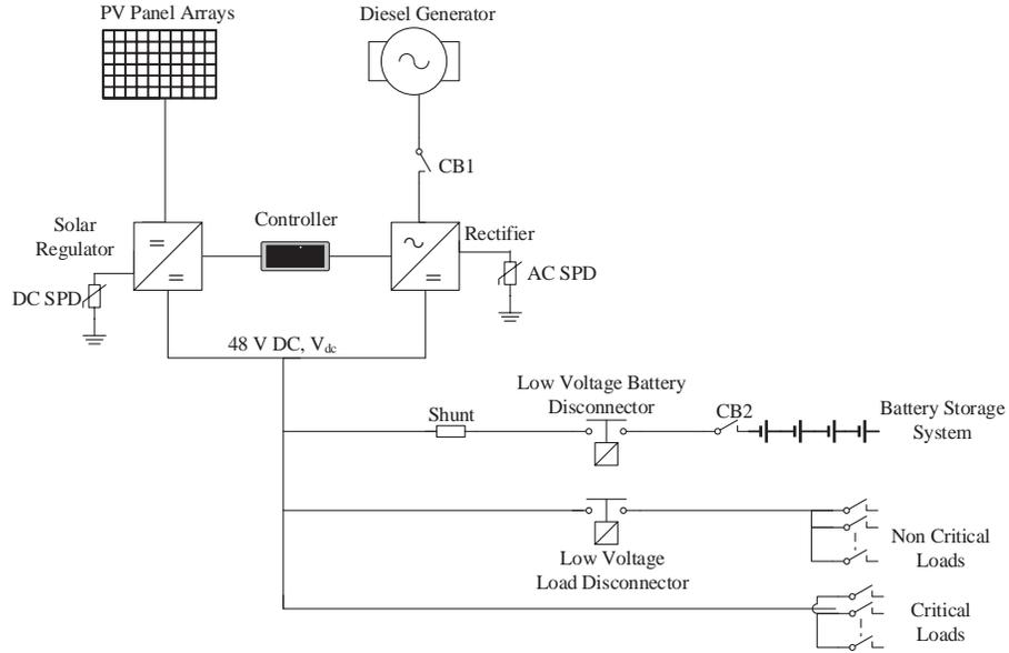
Fig. 1. A commercial hybrid DC microgrid system
