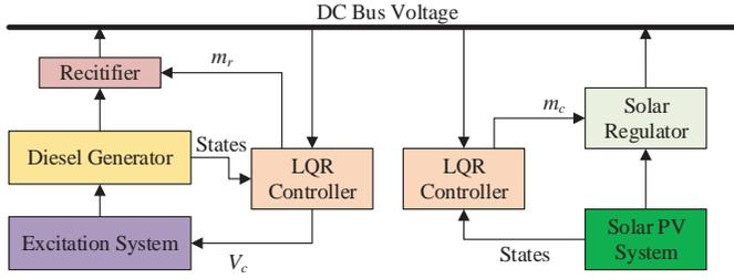
Fig. 6. Block diagram: implementation of LQR controllers for diesel generator and solar PV system
