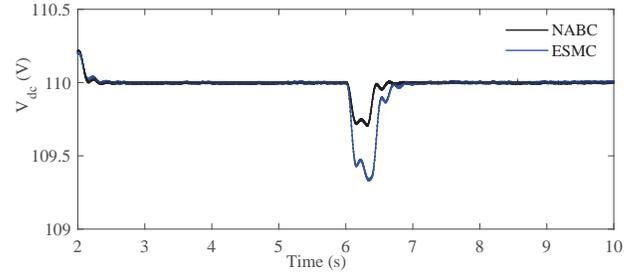
Fig. 6. DC bus voltage in the microgrid under changing of solar irradiance while charging and discharging the BESS
