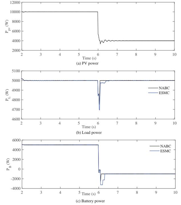
Fig. 5. Power in the DC microgrid under changing of solar irradiation while charging and discharging the BESS
