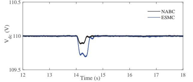
Fig. 9. DC bus voltage in the microgrid under changing load demand while supplying power by the diesel generator
