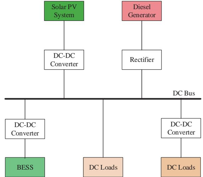
Fig. 1. DC microgrid with BESS and diesel generator
