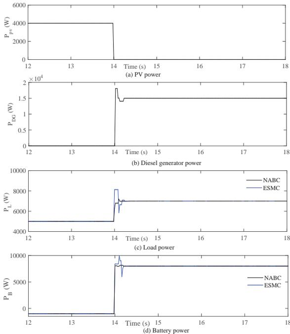
Fig. 8. Power in the microgrid under changing load demand while supplying power by the diesel generator
