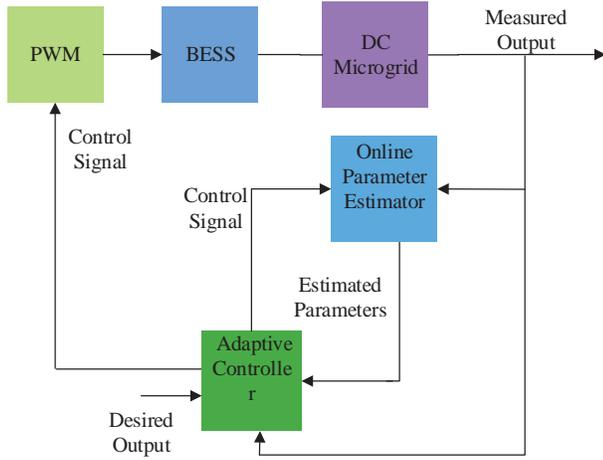
Fig. 4. Implementation block diagram of the adaptive backstepping controller for the BESS
