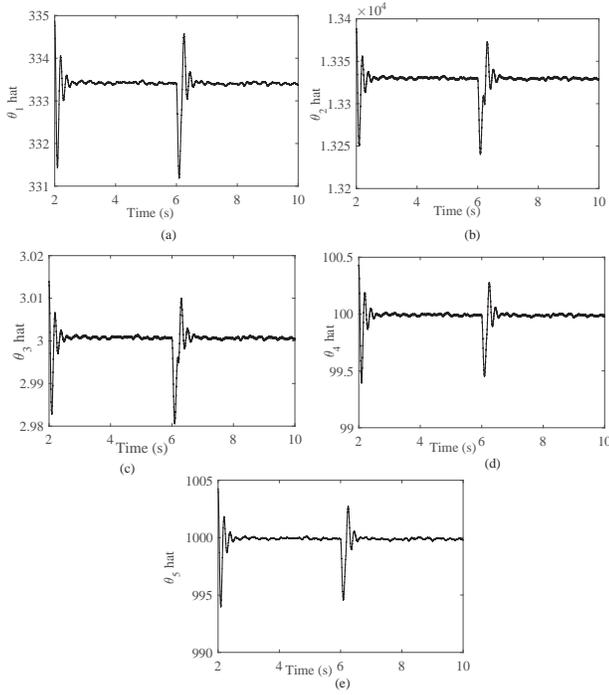
Fig. 7. Estimated parameters of the BESS with the DC-DC converter under changing of solar irradiance while charging and discharging the BESS
