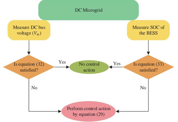
Fig. 3. Control actions by monitoring SOC of BESS and DC bus voltage
