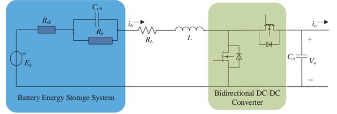
Fig. 2. BESS with bidirectional DC-DC buck-boost converter
