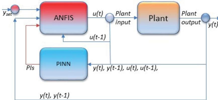
Fig. 3. PI-based ANFIS control system
