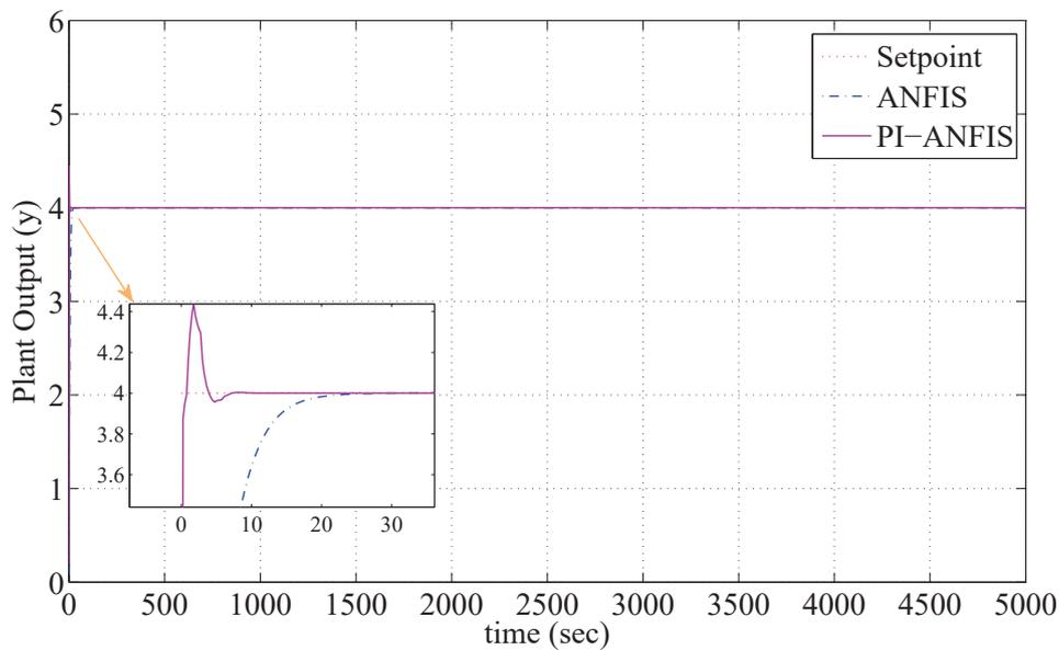
Fig. 5. Constant setpoint tracking using PI-ANFIS and traditional ANFIS controller
