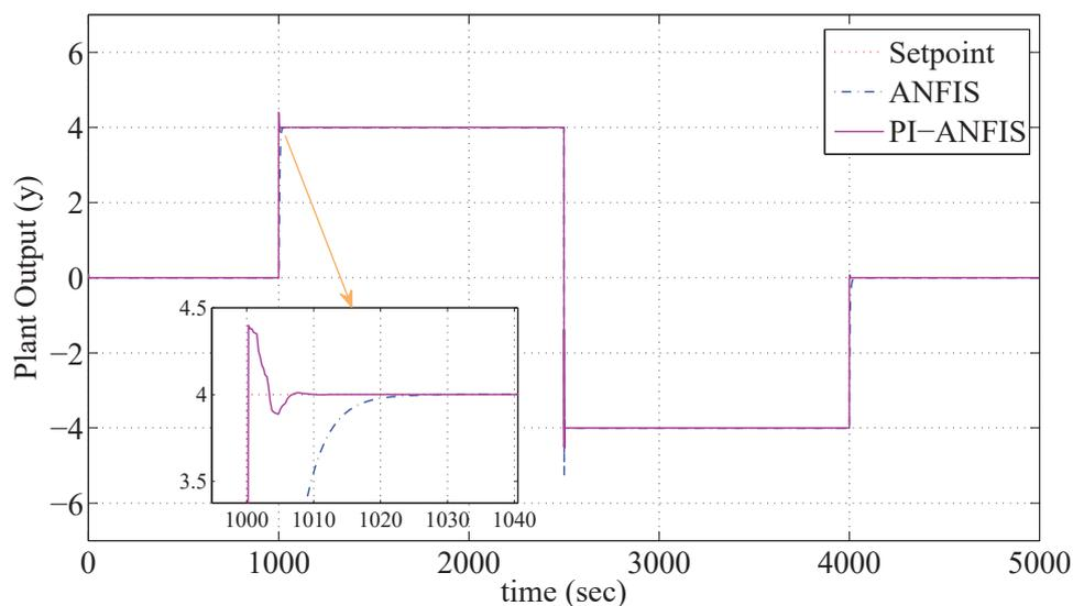
Fig. 7. Step changes setpoint tracking using PI-ANFIS and traditional ANFIS controller
