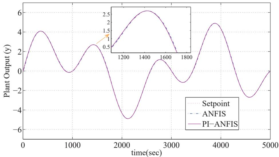
Fig. 6. Wavy setpoint tracking using PI-ANFIS and traditional ANFIS controller
