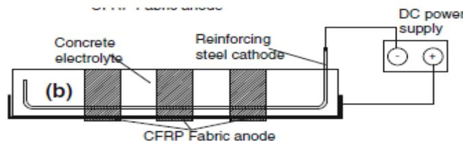
Figure 2 Schematic ICCP application to corroded reinforced concrete beams [24]
