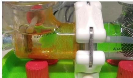
Figure 4 – appearance of a cathode chamber after one week testing under CP= -0.85 V
