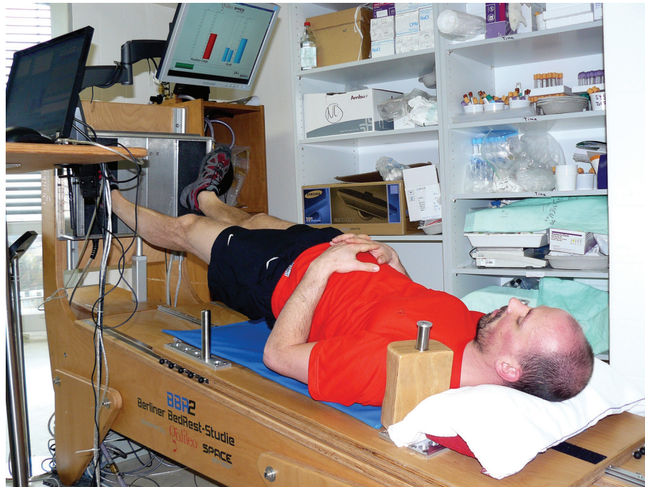
Figure 1. Countermeasure exercise training. Both the resistance exercise only (RE) and resistance exercise with whole-body vibration (RVE) groups performed their exercises on the specially designed Galileo Space exercise device. Subjects were positioned in head-down tilt on a moveable platform with shoulder pads and hand grips preventing downward movement and permitting application of force via the platform. A pneumatic system (not shown) generated the force, applied through the moveable platform, against which the subject needed to resist and move (via the shoulder pads and hand grips). The feet were positioned either side of a platform which could be set to vibrate in the RVE group. Subjects were given visual feedback of their actual and target position in the exercise via a monitor placed in the subjects' field of view. Here the subject is performing the combined back lift and ankle dorsiflexion exercise.
