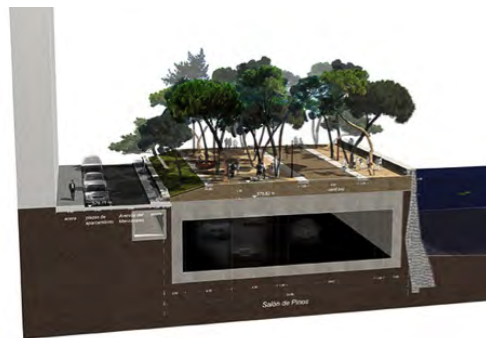
Figure 5.17: Madrid Rio. Indicative planting and public domain over section of the 43km of tunnel. Image: West 8.
