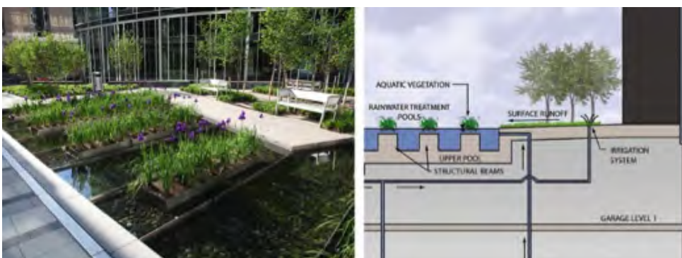
Figure 6.19: Showing scenario 2, horizontal planting and parking garage (includes water recycling system). Sasaki Associates (image: Eric Taylor), The Avenue, USA.
