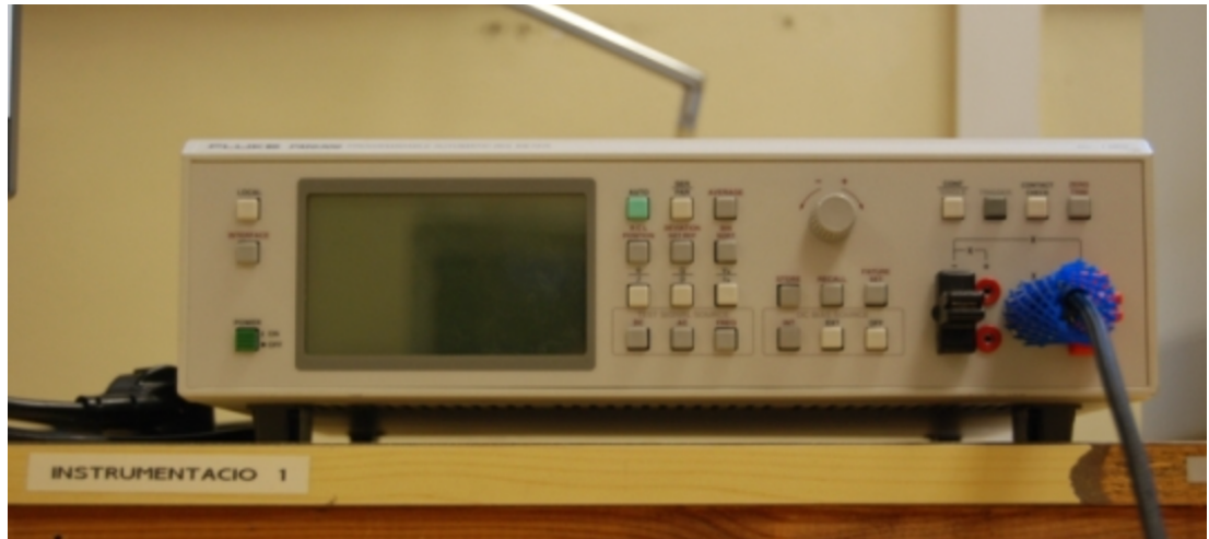
Figure 3.5 PM 6306 LCR Meter
