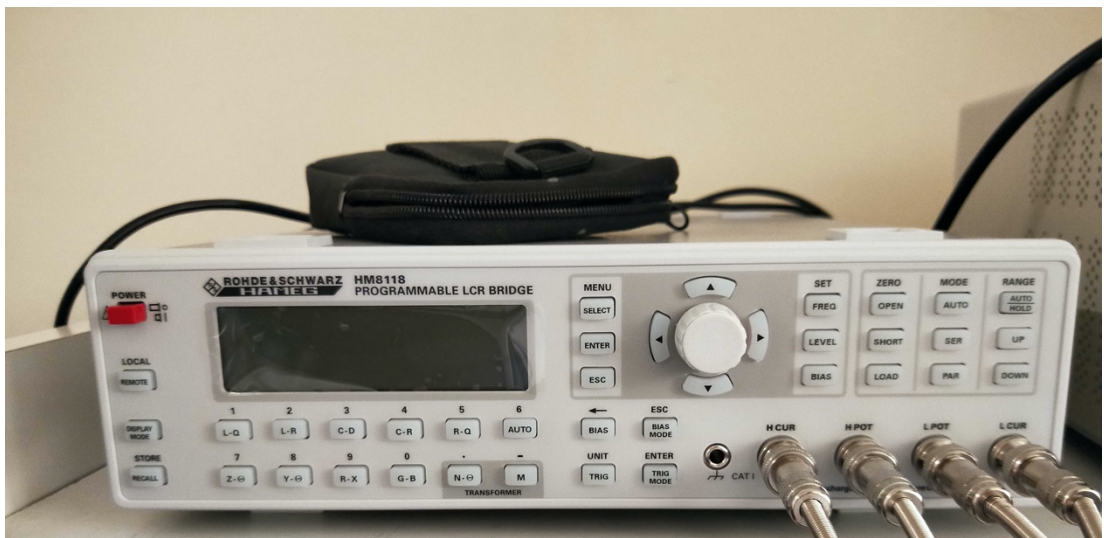
Figure 3.4 HM8118 LCR Meter
