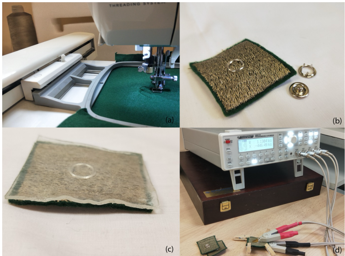
Figure 4.1 Fabrication and experimental process: (a) embroidery setup, (b) sample e-textile electrode prepared with snap, i.e., ball and spiked ring components (c) e-textile electrode with hydrogel pad tested as a wet e-electrodes, and (d) LCR meter with frequency setting 50 kHz [47]. “© IOP Publishing. Reproduced with permission. All rights reserved.”
