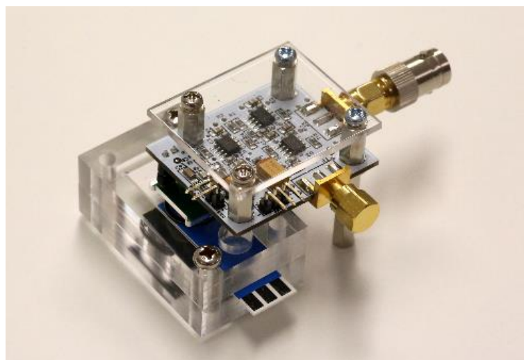
Figure S4.11. Photograph of the cell holder containing magnet and Zensor SPE, coupled with the silicon photomultiplier detector (ASD-RGB3S-P; AdvanSiD, Italy) and ASD-EP-EB-N amplifier board (AdvanSiD).
