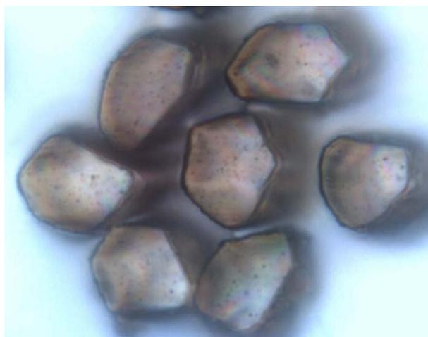
Fig. 6. Cross sectional microscopy of the PPy coated plasma treated PET fibers.
