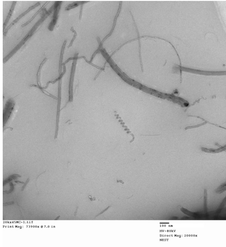
**Figure 2:** TEM image of the MWNTs/PVA nanofibers treated by methanol/crosslinking.
