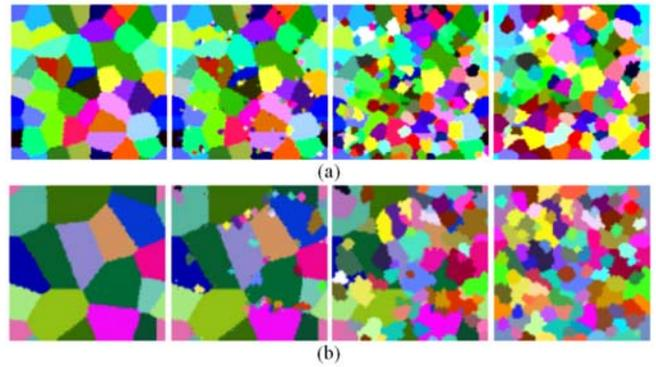
**Figure 22.** comparison two final microstructure when the initial grain size in different.  $d_0=20\text{ }\mu\text{m}$  (a),  $d_0=35\text{ }\mu\text{m}$  (b).
