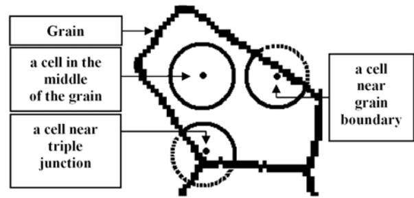
**Figure 17.** Three cells in different positions, into the grain, near grain boundary and close to the triple junction.
