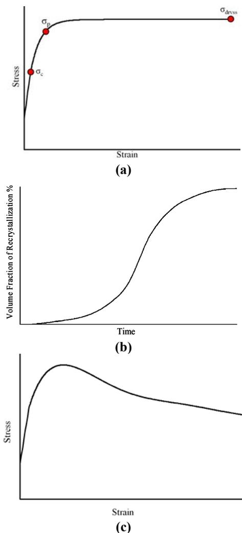
**Figure 8.** Schematic dynamic recovery curve (a), typical “S” shape of volume fraction percentage of recrystallized microstructure (b), Schematic dynamic recrystallization curve (c).
