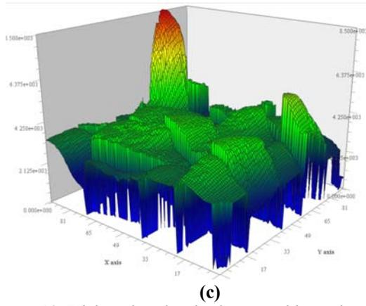
**Figure 18.** Dislocation density increased in each grain during deformation and a dislocation gradient was demonstrated in each grain.
