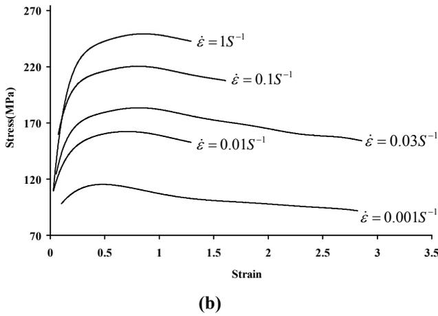
**Figure 3.** Stress-strain curves from torsion test at (a) constant strain rate ( $0.01S^{-1}$ ) and (b) at constant temperature ( $900\text{ }^{\circ}C$ ).
