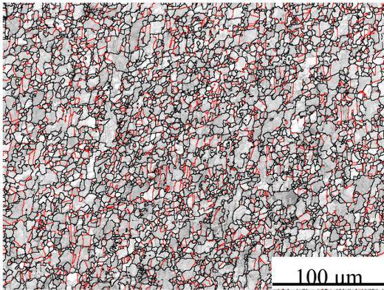
**Figure 21.** Microstructure from hot torsion test in  $T=900\text{ }^{\circ}\text{C}$ ,  $\dot{\epsilon}=0.01\text{ S}^{-1}$
