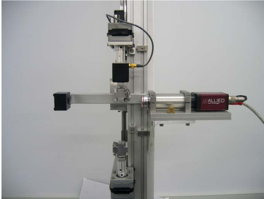
(a). The clamps and camera system of SIFAN3001
