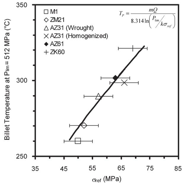
Fig. 14—The billet temperature at the 512 MPa pressure limit vs  $\sigma_{\text{ref}}$ . In this case  $k=0.154$ . (Error bars are estimates of the range based on repeat tests.)
