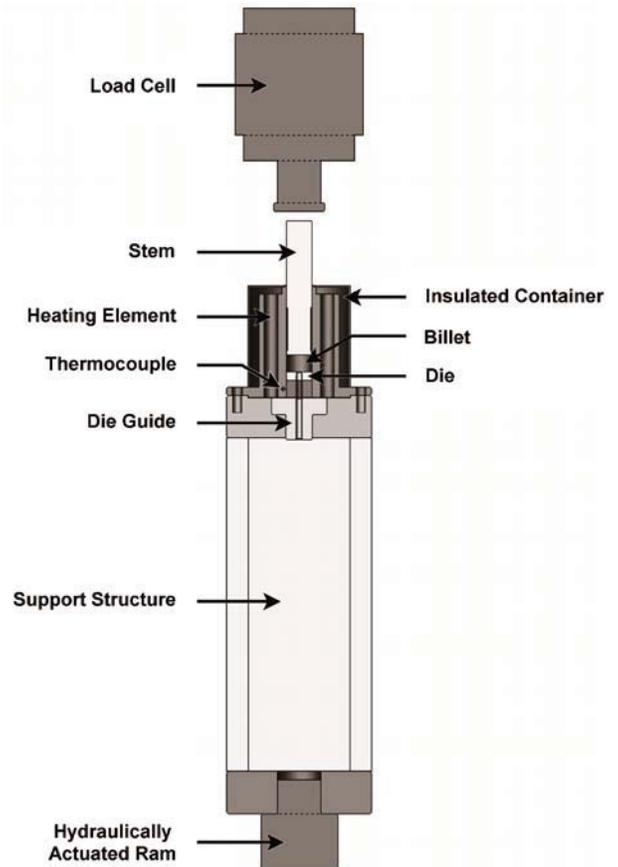
Fig. 2—Sectioned schematic representation of the extrusion rig.
