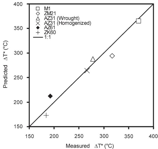
Fig. 16—The  $\Delta T^*$  predicted from Eq. [11] vs the  $\Delta T^*$  measured from the extrusion limit diagrams.
