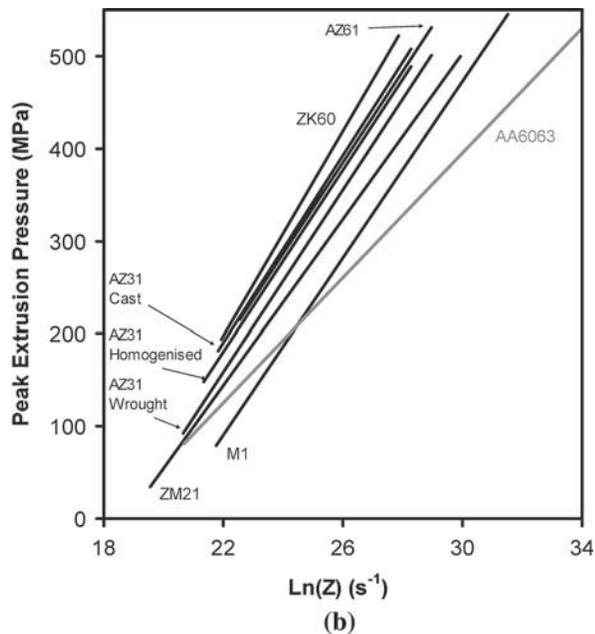
Fig. 4—Influence of the Zener-Holloman parameter on the peak pressure: (a) AZ31 (homogenized) and (b) summary of trends.
