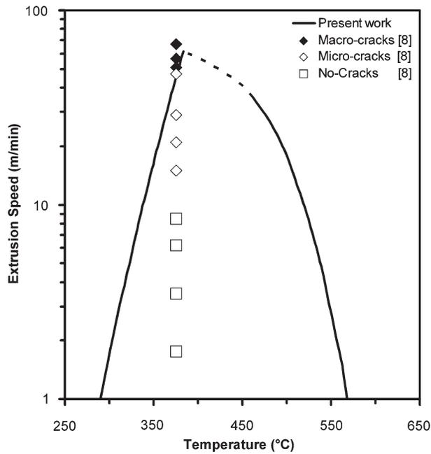
Fig. 10—Wrought AZ31 billet extrusion limits compared with the cracking limit identified by Sillekens.<sup>[8]</sup>
