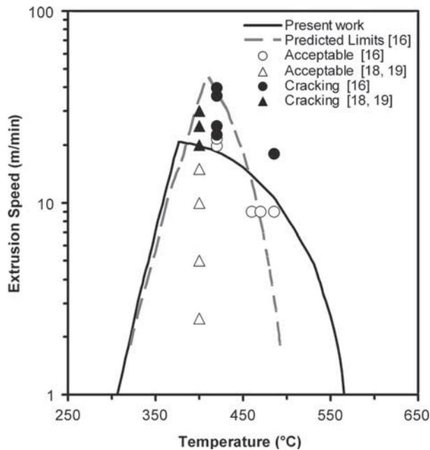
Fig. 11—As-cast AZ31 billet extrusion limits compared with the cracking limits identified by Barnett *et al.*<sup>[16]</sup> and Murai *et al.*<sup>[18,19]</sup>
