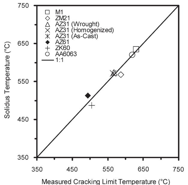
Fig. 15—Solidus temperature vs the cracking limit temperature at a  $V_E$  of 1 m/min.
