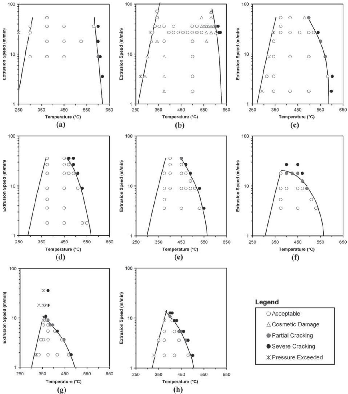
Fig. 7—Extrusion limit diagrams for the present study. The left (pressure) limit was determined using empirical model extrapolation. The right (cracking) limit is a curve fitted through the partial cracking data: (a) homogenized AA6063, (b) wrought M1, (c) wrought ZM21, (d) wrought AZ31, (e) homogenized AZ31, (f) as-cast AZ31, (g) wrought AZ61, and (h) homogenized ZK60.
