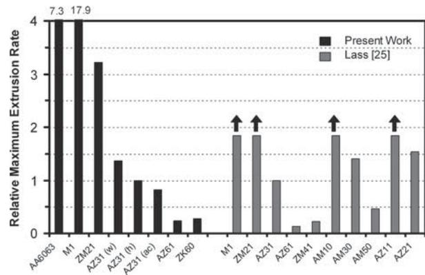
Fig. 12—Maximum extrusion speed of present and published alloys relative to homogenized AZ31 magnesium billet (AZ31 alloy = 1).
