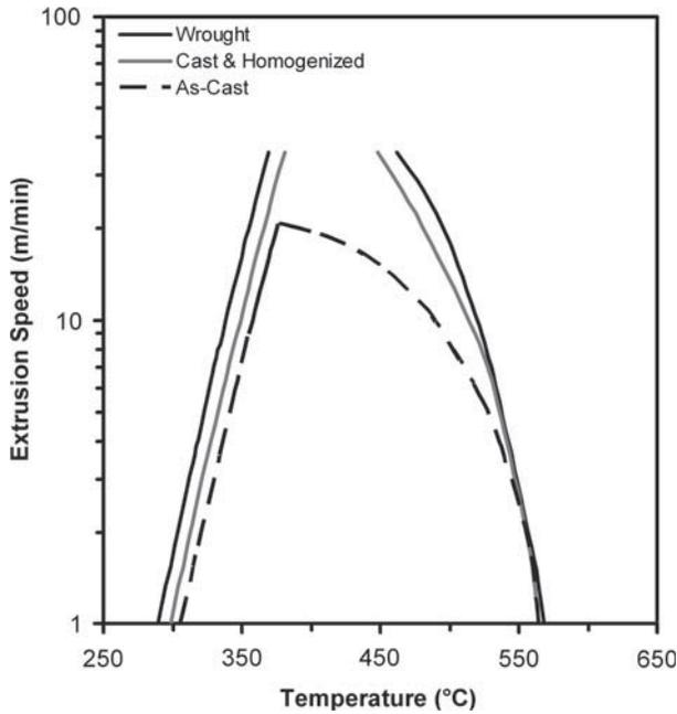
Fig. 8—Effect of billet condition on the extrusion limits of AZ31 (pressure limit: 512 MPa).
