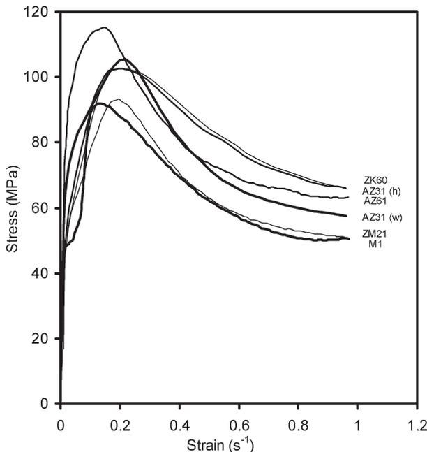
Fig. 13—Flow curves from uniaxially compressed billet material at 350 °C, 1 s<sup>-1</sup> (AZ31 data taken from<sup>[31]</sup>).
