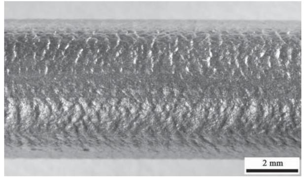
Fig. 6—An example of the surface obtained in the present work for M1 billet showing the orange peel defect (extruded at  $V_R$  15  $\text{mm s}^{-1}$  at 582 °C).
