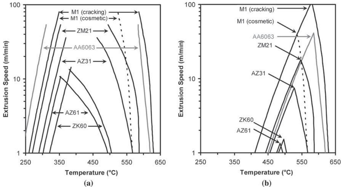
Fig. 9—Collated extrusion limit diagrams: (a) 512 MPa pressure limit and (b) 190 MPa pressure limit.
