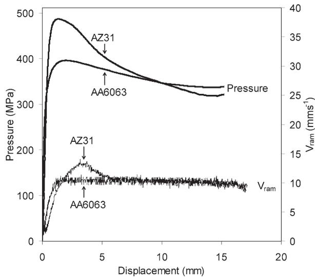
Fig. 3—Typical pressure-displacement trace with corresponding ram speed for homogenized AZ31 and AA6063 billet at an initial billet temperature of 375 °C.
