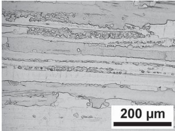
Fig. 1—Microstructure of the M1 billet.
