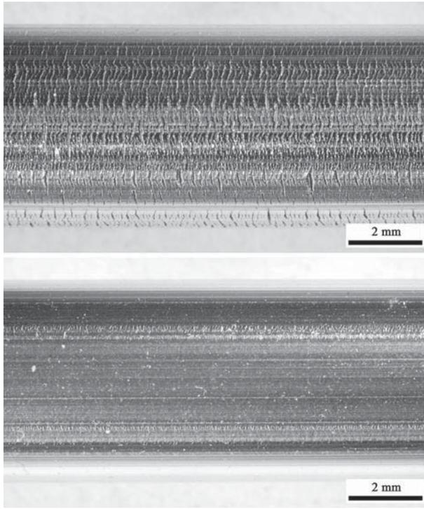
Fig. 5—Examples of the surfaces obtained in the present work for homogenized AZ31 billet extruded at 490 °C, at  $V_R$  10  $\text{mm s}^{-1}$  (top) and 7  $\text{mm s}^{-1}$  (bottom).
